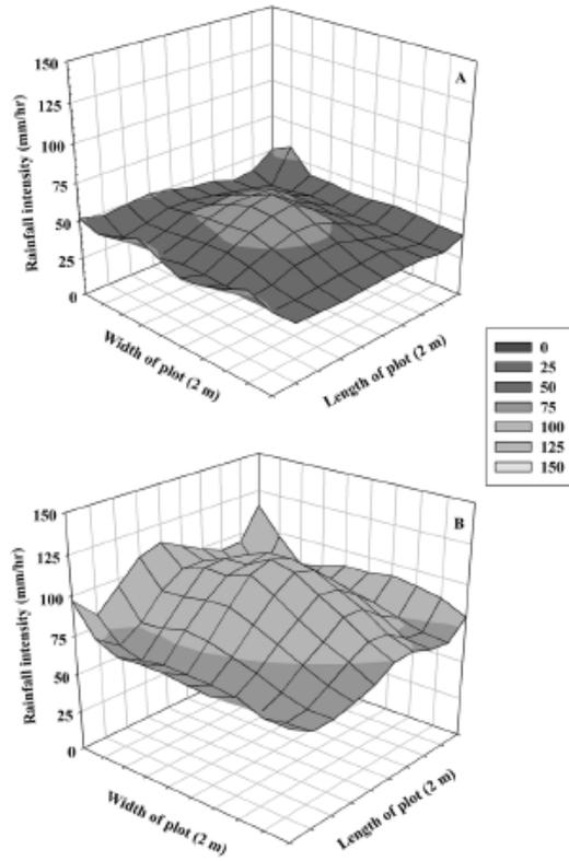
Figure 3. The rainfall intensity distribution of simulated rainfall collected over the 2- × 2-m sample area (5-min duration) for the (A) Fulljet 3/8HH-SS24 WSQ nozzle (CU = 86%) and (B) Fulljet 1/2HH-SS50 WSQ nozzle (CU = 85%) at 34.5-kPa operating pressure.
