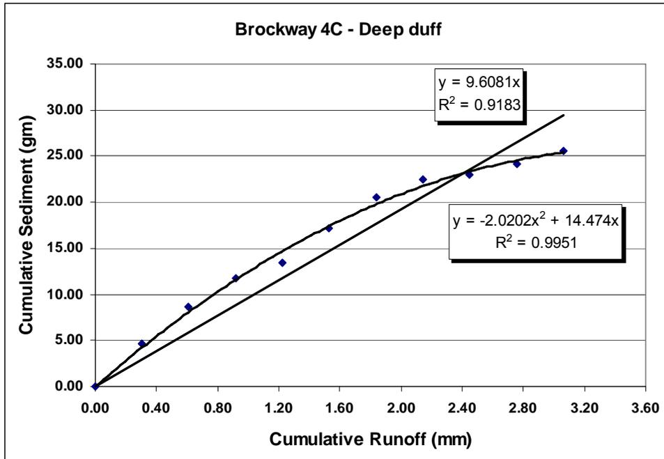
Figure 32. Cumulative sediment as it depends on cumulative runoff from 1 m<sup>2</sup> test plot of Figure 31.
