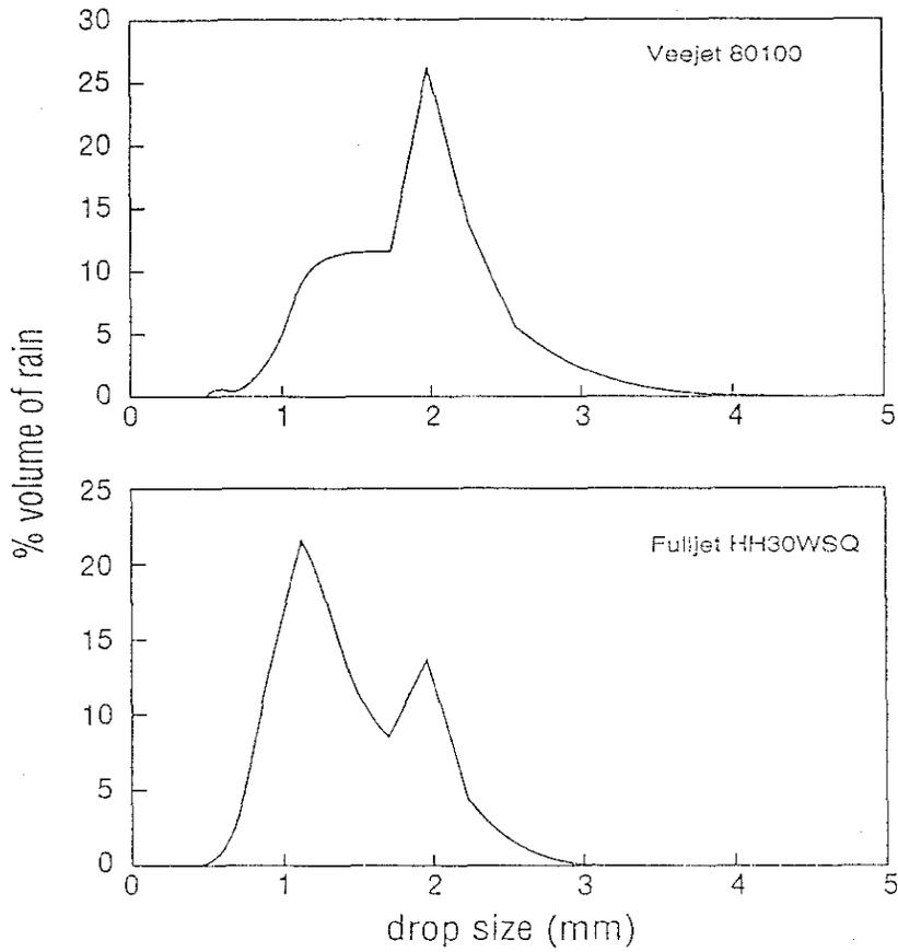
**Figure 22.** Rain drop-size distributions from two commonly used nozzles in RSs, the Veejet 80100 and the Fulljet HH30 WSQ operating at pressures of 50 and 30 kPa, respectively, as tested by Kinnel (1993).
