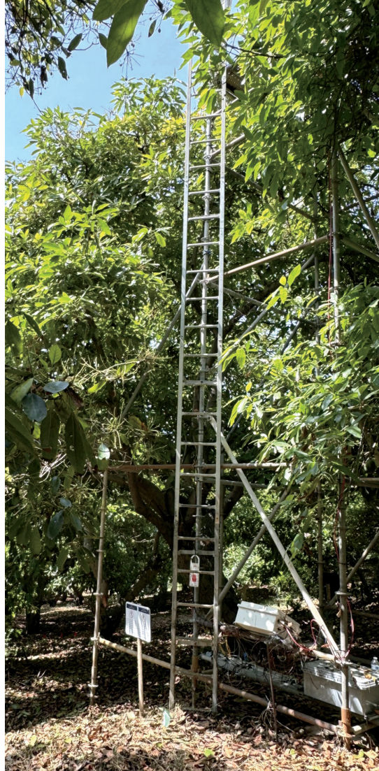
Sensors mounted on towers high above the avocado orchard canopy were crucial in collecting real-world data for more precise crop coefficients. Photo: Ali Montazar.
